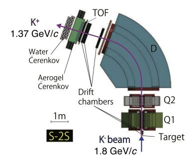
Fig. 9. Schematic view of the S-2S spectrometer system.
