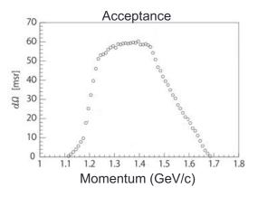
Fig. 10. Acceptance of the S-2S spectrometer as a function of momentum. The momentum for the  $\Xi$ -hypernuclei bound states production corresponds to ~1.37 GeV/*c*.
