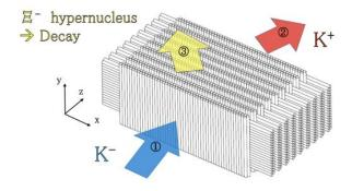
Fig. 15. A conceptual design of the active target made of  $\phi$ 3 mm scintillation fibers.
