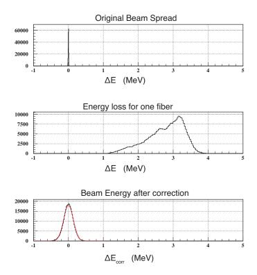
**Fig. 16.** Results of the RCNP test run for the fiber scintillator. Top) Beam energy spread of 65-MeV proton beam, Middle) Energy loss distribution measured with the Grand Raiden spectrometer for a  $\phi$ 3 mm scintillating fiber (Widely distributed due to energy loss position dependence and straggling.), Bottom) After correction by using the fiber light output. The width gets narrower.
