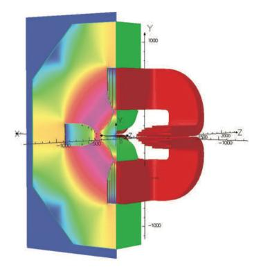
Fig. 13. Simulated magnetic-field map of the Q1 magnet of the S-2S spectrometer system.
