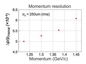
Fig. 11. Momentum resolution of the S-2S spectrometer in FWHM assuming that the position resolution of the tracking detectors are  $250 \,\mu$ m in r.m.s. as a function of momentum.
